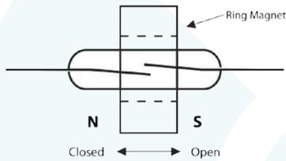
A reed switch moving through a circular/ring magnet will operate up to 3 times.
