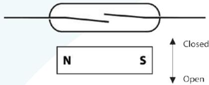
A magnet moved in a front to back motion (perpendicular towards and away) will operate the reed switch
