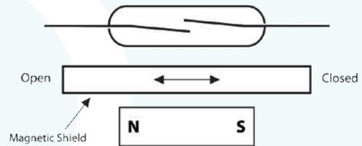
**Shielding (Indirect Actuation):**
